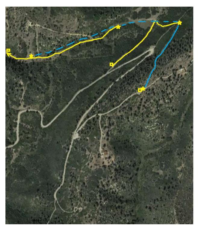
Yellow lines are power wires. Yellow squares are electrical meters. Yellow stars are electrical equipment.
